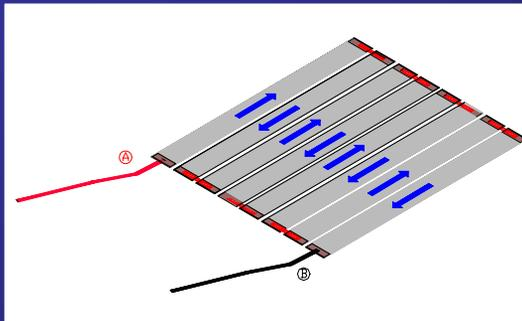
$$R_T = 1 \frac{\Omega}{\text{strip}} \times 8 \text{ strips} = 8 \Omega$$
