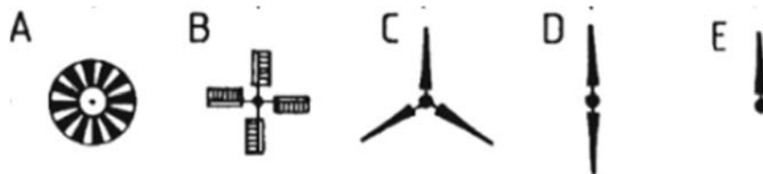
Figure 4. Five blade configurations with different torque characteristics: (A) American, (B) 4-Blade, (C) 3-Blade, (D) 2-Blade, and (E) 1-Blade. Torque models for each configuration emphasize blade count rather than geometry.
