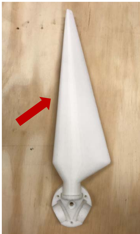
Figure B-1. 3D printed blade inserted into bottom-rotor hub.
