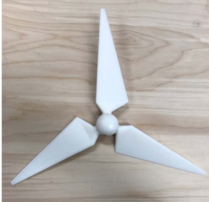
Figure B-2. Top-rotor hub securing the blades in place.
