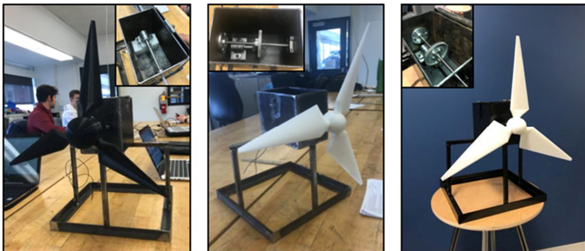
Figure 2. Sequence of prototypes for our team's small-scale wind turbine: (left) alpha 1 prototype, (center) alpha 2 prototype, and (right) beta prototype.
