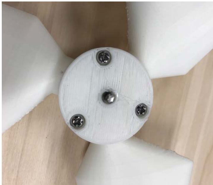
Figure B-3. Rotor-hub fastened with screws.
