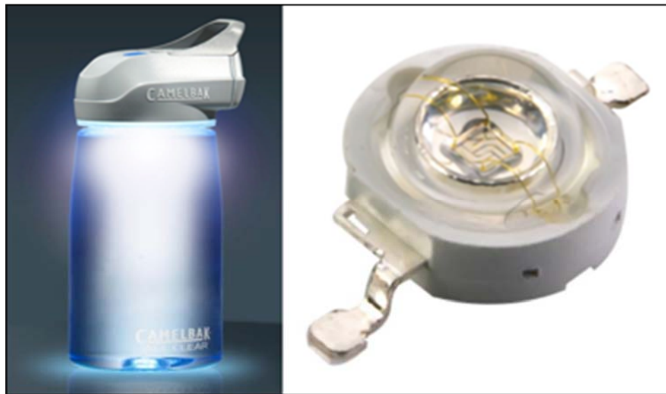
Figure 1. Water container that uses a UV-LED light attached to the inside of the lid [5,6]. The UV-LED light takes just 60 seconds to disinfect a container of water.
