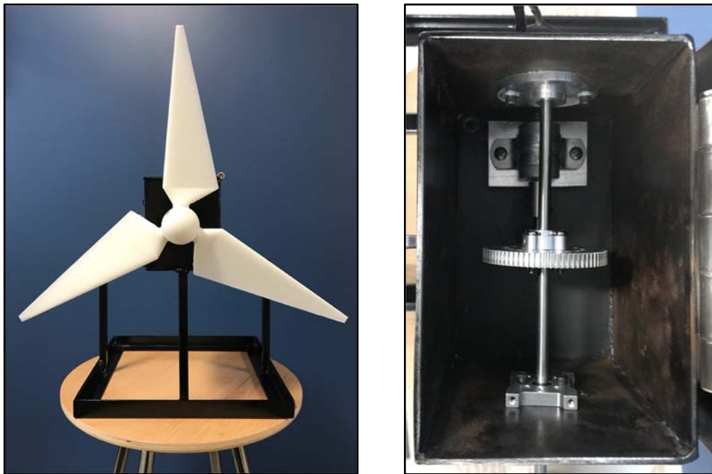
Figure 3. Final design of our wind turbine: (right) 3D printed blades and welded support structure and (left) bearings, shafts, spur gears, machined coupler, and generator in the nacelle.
